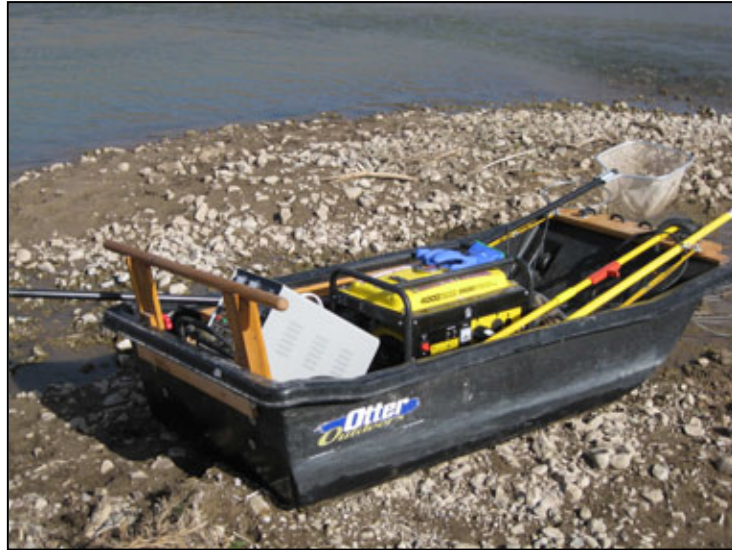
Photo 1. The electrofishing "barge" ready to use.
